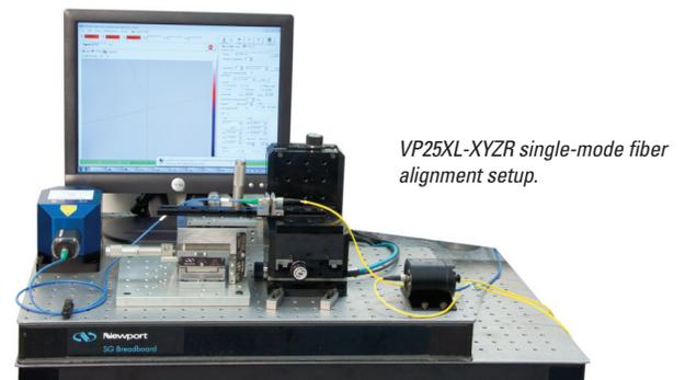
VP25XL-XYZR single-mode fiber alignment setup.
