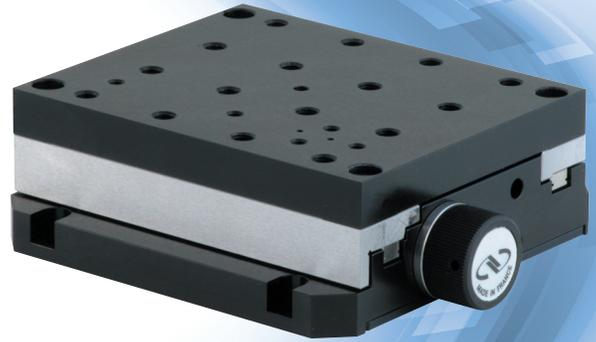
Featuring an aluminium body in a compact package, the VP-25X series has 25 mm travel with exceptional MIM and position stability. Similar to other families of linear stages, the VP-25X also features recirculating ball bearings, a backlash-free ball screw, and a linear steel scale. Applications include: fiber alignment, bio-medical, semiconductor and high precision test and measurement.
